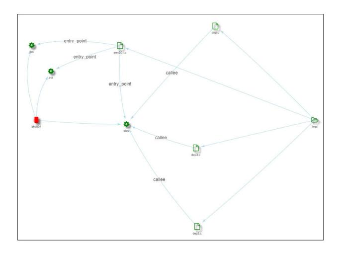
The code implementation of pkg.tst002.swc001.bhv001 has three entry point functions: foo, init and step. All three functions are defined in the file swc001.c. These entry-point functions call other functions defined in the files dep.c, dep2.c and dep3.c.
