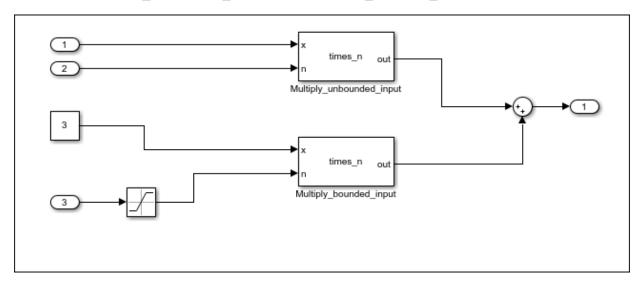
When you analyze custom code, in this case the function times\_n, the analysis shows that an operation in the custom code can overflow. From the analysis results, you can determine that the overflow occurs only when the function is called in the Multiply\_unbounded\_input block but not when it is called from the Multiply bounded input block.
